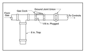
Figure 1: Recommended Piping to Controls
